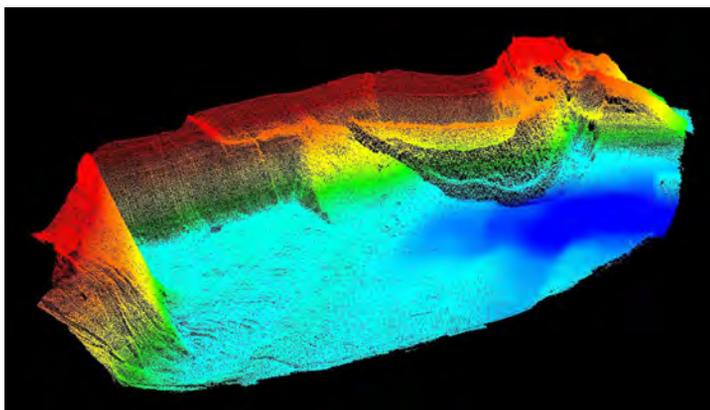
Approach Channel Acceptance Survey – Multibeam point cloud of upstream approach channel & spur dike, perspective view
