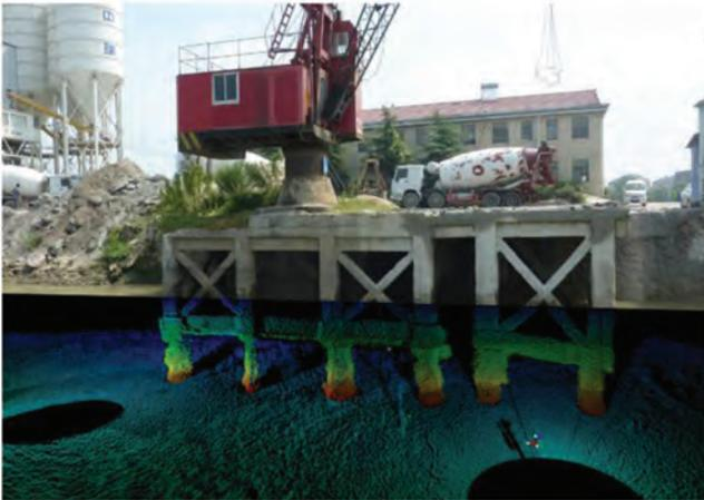
**Figure 6:** BlueView construction monitoring data image
