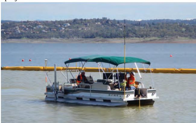
Approach Channel Acceptance Survey – Survey vessel acquiring multibeam sonar data
