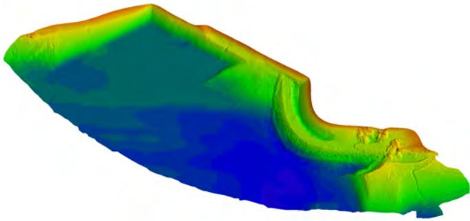
Approach Channel Acceptance Survey – Multibeam TIN model of upstream approach channel & spur dike, perspective view
