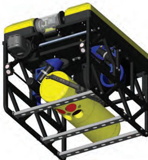
**Figure 6b:** outfitted with AUV payload modules
