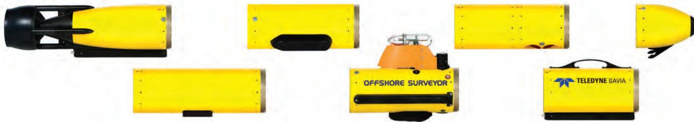
Figure 2: The Gavia modules are fully independent and interchangeable
