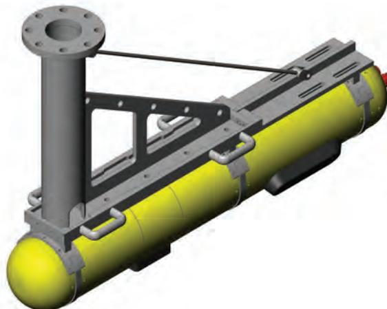
**Figure 7:** AUV payload modules pole mounted from a vessel of opportunity
