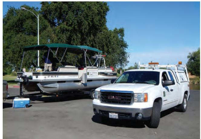
Survey Vessel – 24' Fisher pontoon configured for multibeam & mobile LiDAR acquisition
