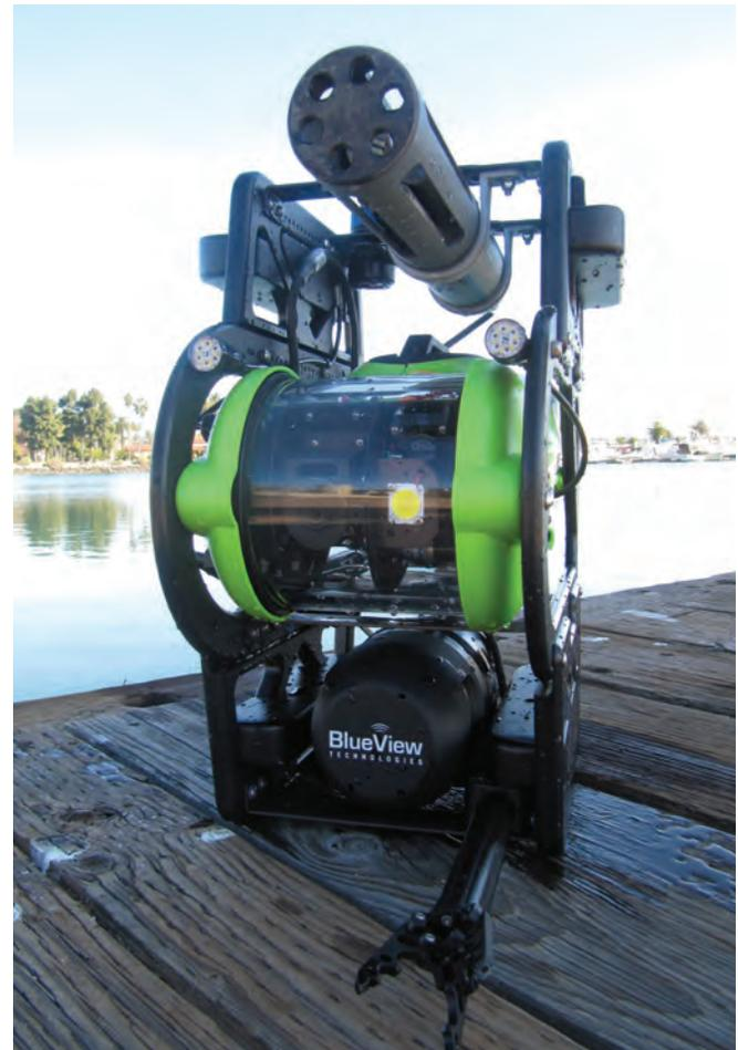
**Figure 8:** SeaBotix LBV200 with BlueView P900-130 imaging sonar
