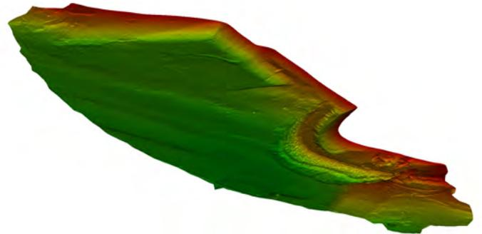
Approach Channel Acceptance Survey – Multibeam TIN model of upstream approach channel & spur dike, perspective view
