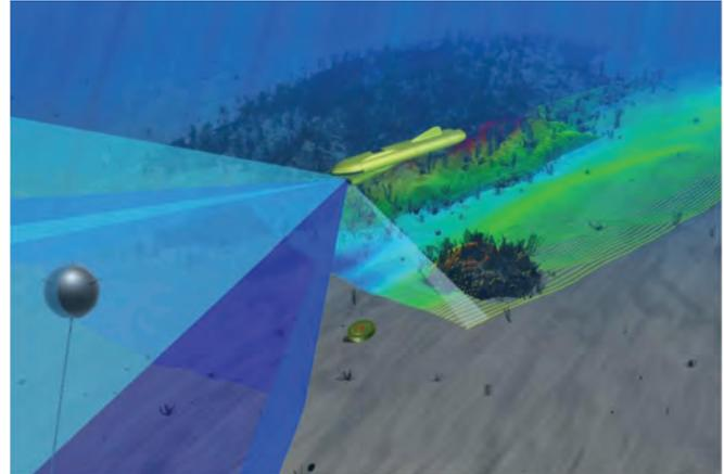
**Figure 7:** BlueView forward looking sonar, micro-bathymetry and gapfil sonar on AUV
