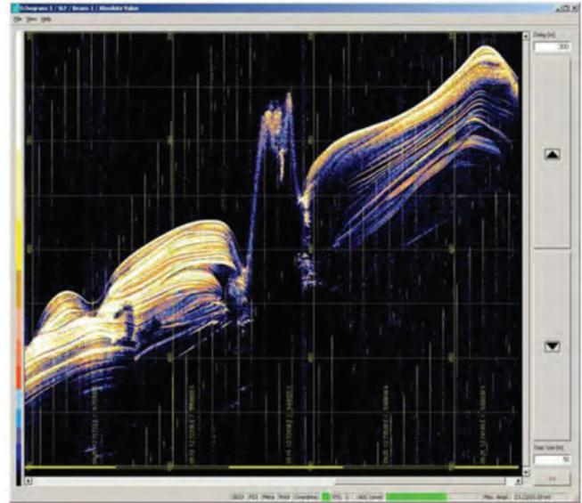
**Figure 4:** More than 50m penetration along a slope at approx. 400m water depth. Courtesy of University of Bremen, recorded onboard research vessel Meteor
