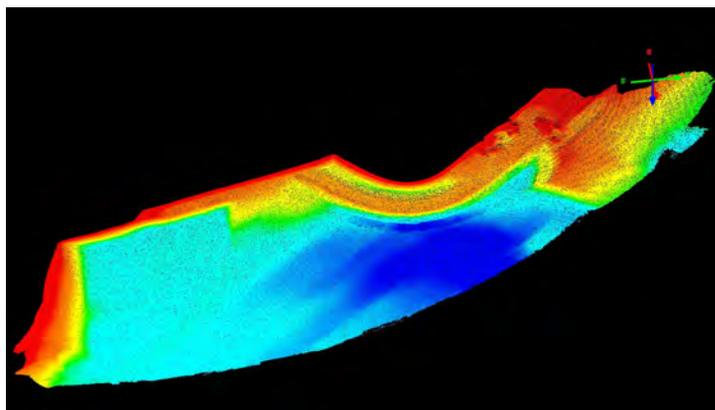
Approach Channel Acceptance Survey – Multibeam point cloud of upstream approach channel & spur dike, plan view
