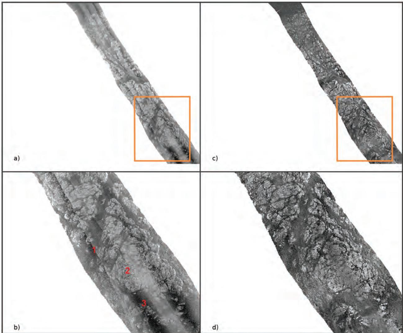
**Figure 2:** Results from the Shallow Survey 2015 dataset. a) raw mosaic (dB), b) zoom on the raw mosaic, c) fully compensated mosaic (dB), d) zoom on the fully compensated mosaic. The contrast of the mosaics were adjusted, removing 1% outliers, for better visualization.
