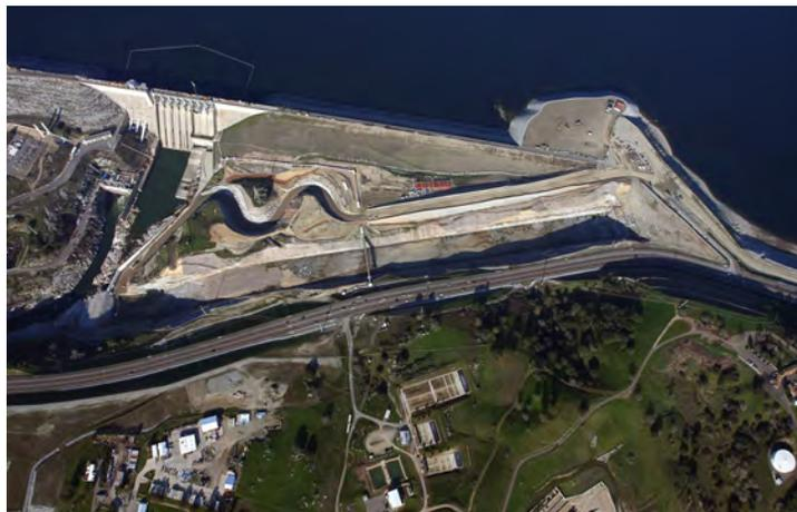
Aerial View – Existing Spillway on left. Auxiliary Spillway and Spillway Chute under construction to the right (©Google Earth)
