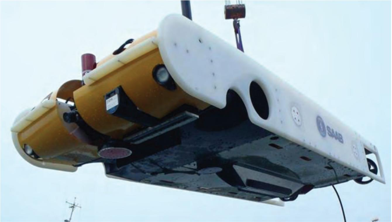
**Figure 3** Sabertooth with the survey sensors installed
