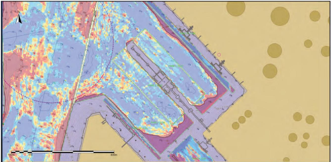
Dredging information based on difference of latest multibeam surveys and maintenance levels
