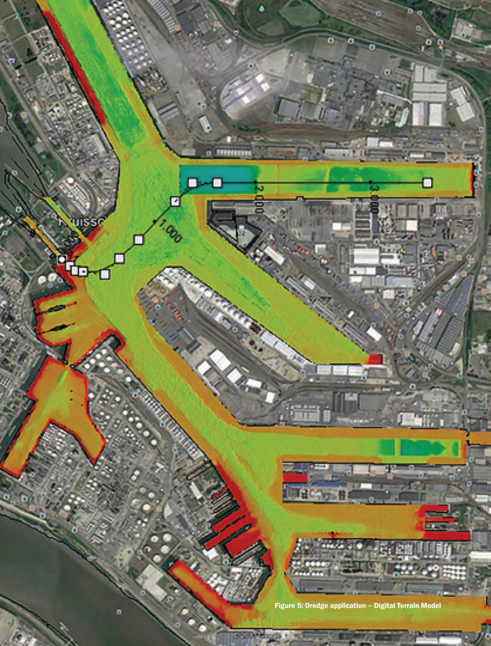
Figure 5: Dredge application - Digital Terrain Model
