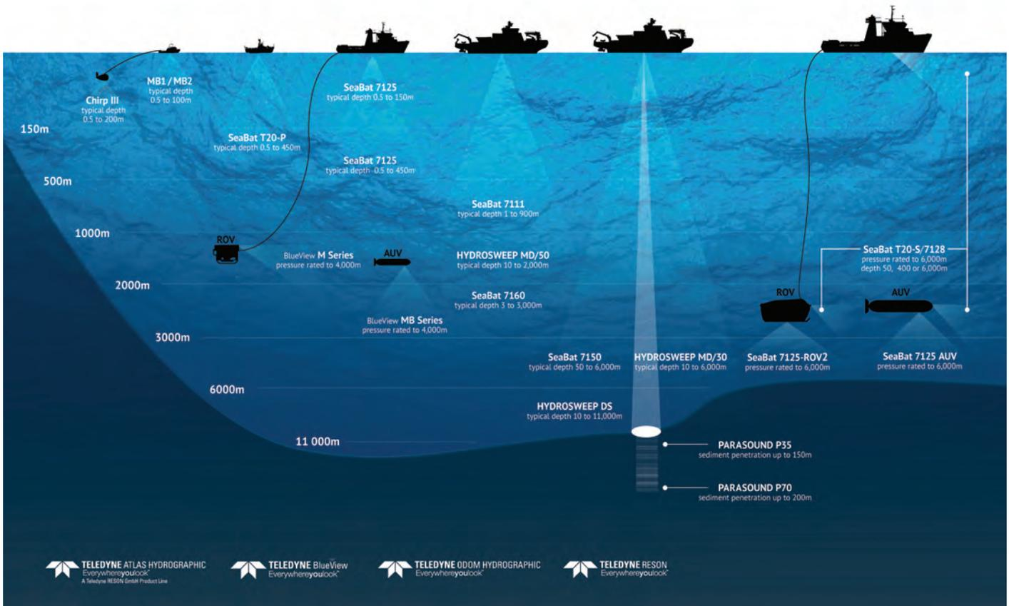
**Figure 3:** Teledyne Marine multibeam echosounder and sonar range overview
