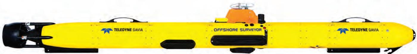
Figure 1: The Gavia AUV
