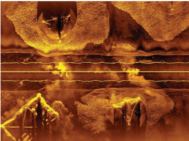
Between the legs of a jack up rig Gavia AUV
