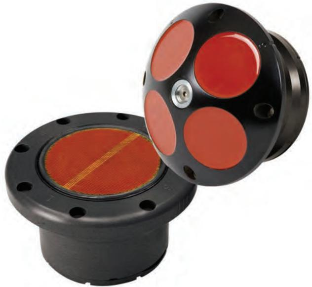
**Fig. 1.** Teledyne RDI's Explorer DVL. This 600 kHz sonar provides navigation for small underwater platforms that require reduced size and weight. Explorer has been used on AUVs, gliders, ROVs, and diver platforms.
