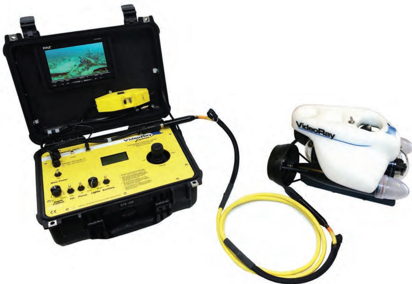
enhanced horizontal and vertical thrusters that increase the submersible's maximum speed to 2.9 knots. The Voyager provides a live video feed from a submerged robotic camera to a topside control panel. The Voyager is depth rated to 250 ft (76 m) and designed for basic underwater visual operations in a low current environment.
