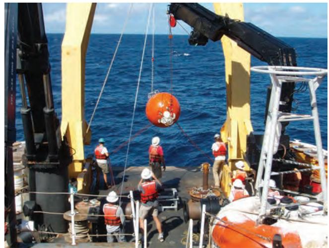
**Fig.1.** Teledyne RD Instruments' 75 kHz Long Ranger ADCP deployment (Rick Cole, RDSEA International)
