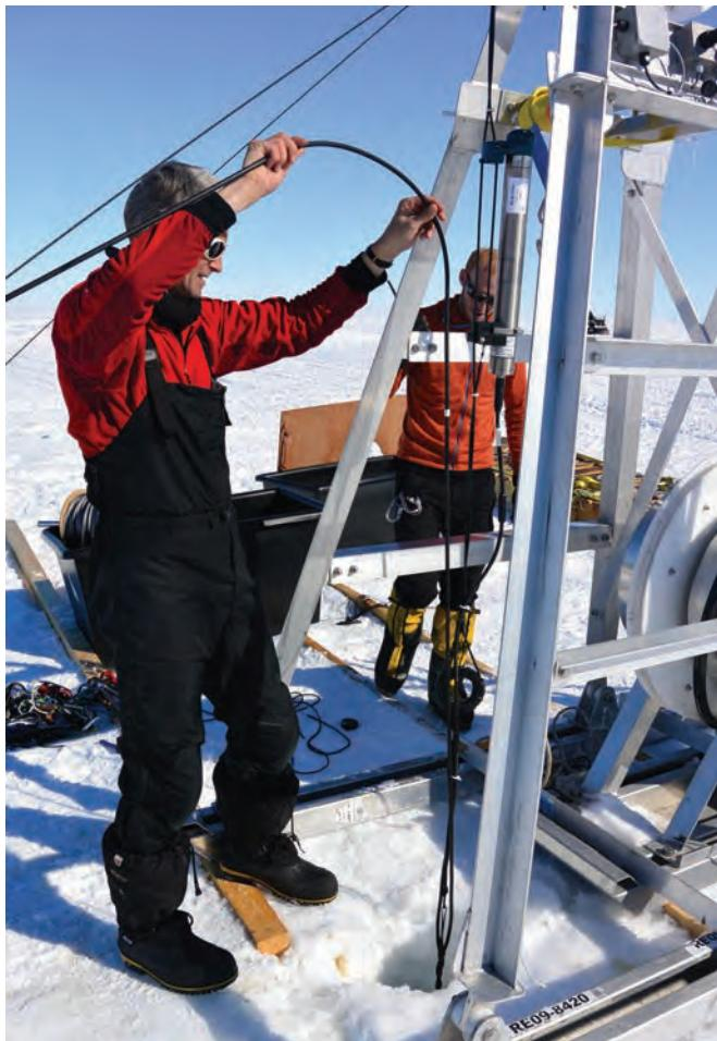
Keith Nicholls attaching the thermistor cable to the main mooring cables.
