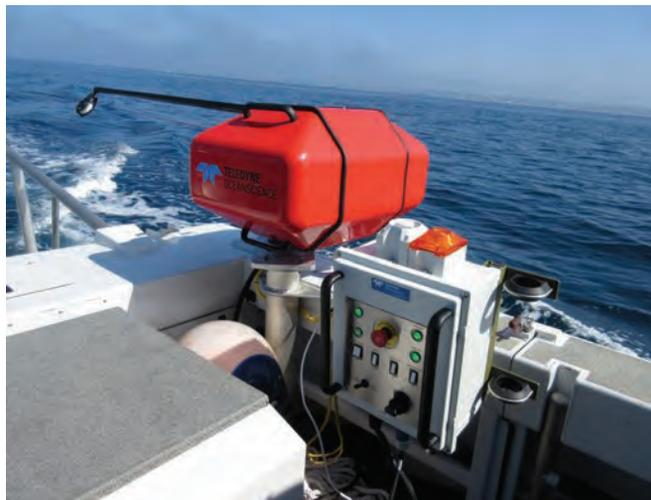
**Fig.6.** Teledyne Oceanscience rapid CAST underway SV probe allows for underway sound velocity measurements
