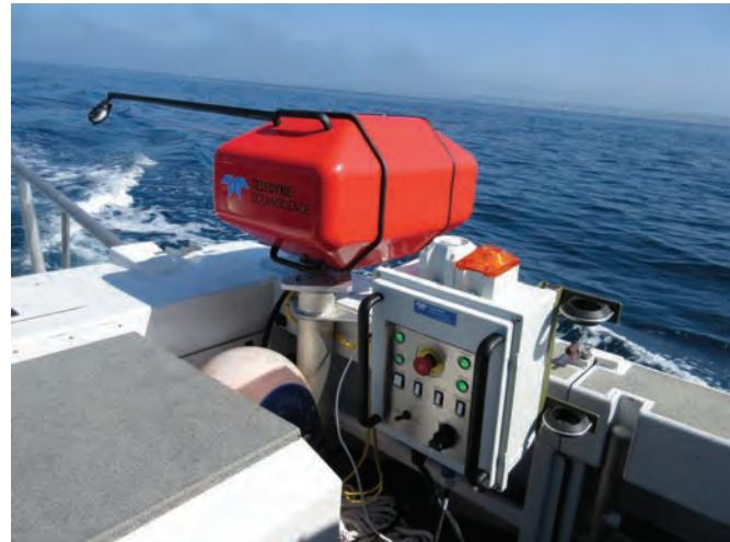
**Fig.6.** Teledyne Oceanscience rapid CAST underway SV probe allows for underway sound velocity measurements
