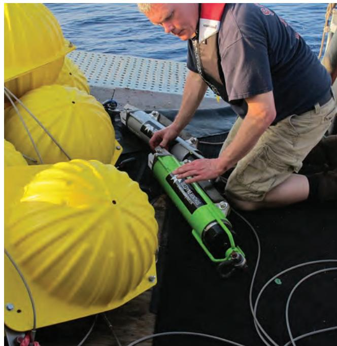
**Fig.7.** Teledyne Benthos's acoustic releases await deployment together with deep-sea glass spheres encased in yellow hard hats
