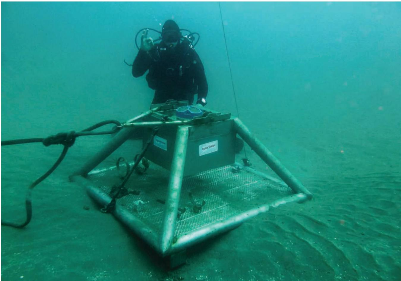
**Fig.5.** Teledyne RDI ADCP installed for seabed deployment
