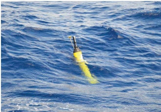
**Fig.2.** Teledyne Webb Research's APEX drifting profiler used to measure subsurface currents and profiles of temperature and salinity.
