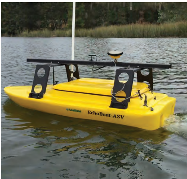
Figure 8 EchoBoat-ASV™ equipped with a SonarMite DFX™ Echosounder, Trimble GA830 GNSS Antenna, and Seafloor AutoNav™
