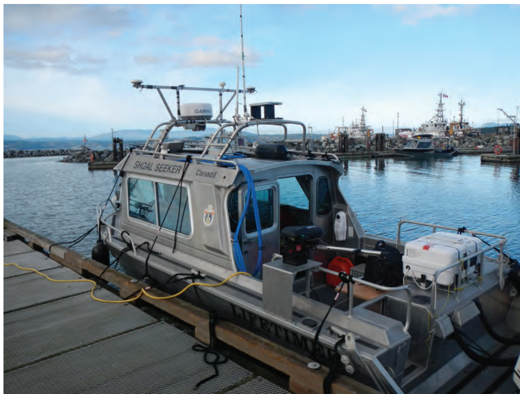
CSL Shoal Seeker. Equipped with an R2Sonic 2022, Applix POS MV and AML Oceanographic Minos X (SVP); the vessel provided an ideal platform for testing CARIS Onboard.
