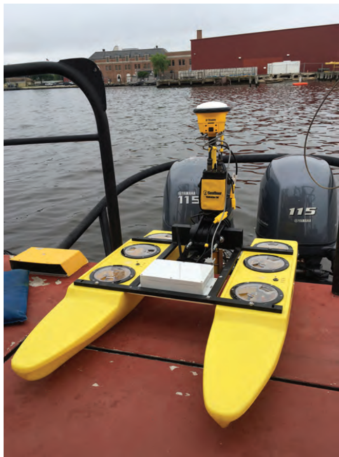
Figure 6 Seafloor Systems HyDrone-RCV integrated with HydroLite-TM, Trimble SPS985 GNSS Smart Antenna, and Seafloor Radio Telemetry System
