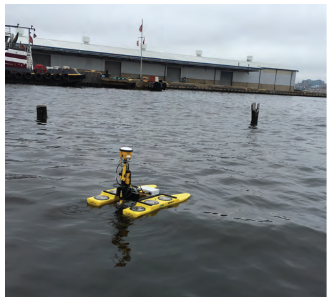
Figure 10 & 11 Remotely controlled HyDrone-RCV surveys the hazard area of submerged dock
