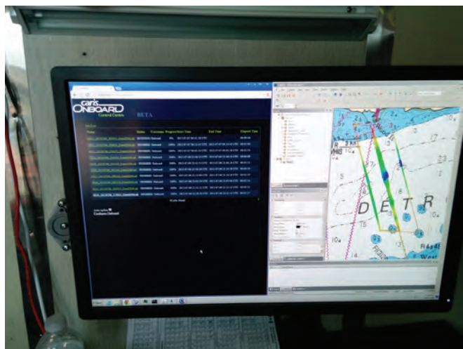
View of CARIS Onboard running on the F.G. Creed. Left on the screen is Control Centre, used for monitoring the processing progress. Right on the screen is CARIS Easy View™ connected to the live updating CUBE surface.
