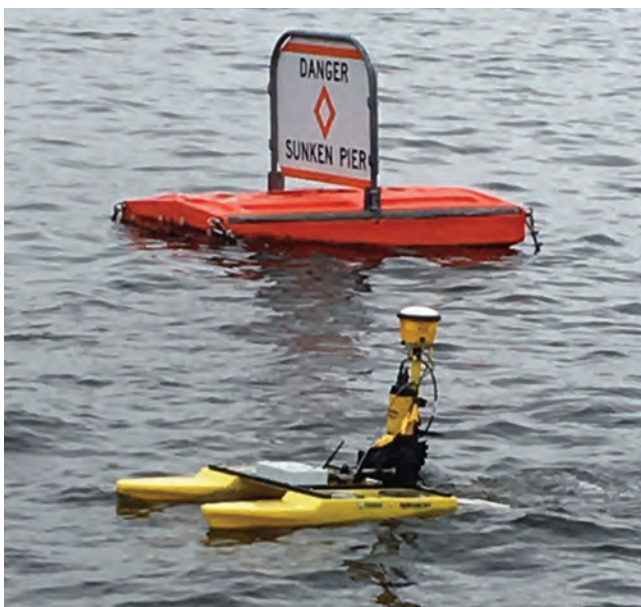
Figure 10 & 11 Remotely controlled HyDrone-RCV surveys the hazard area of submerged dock
