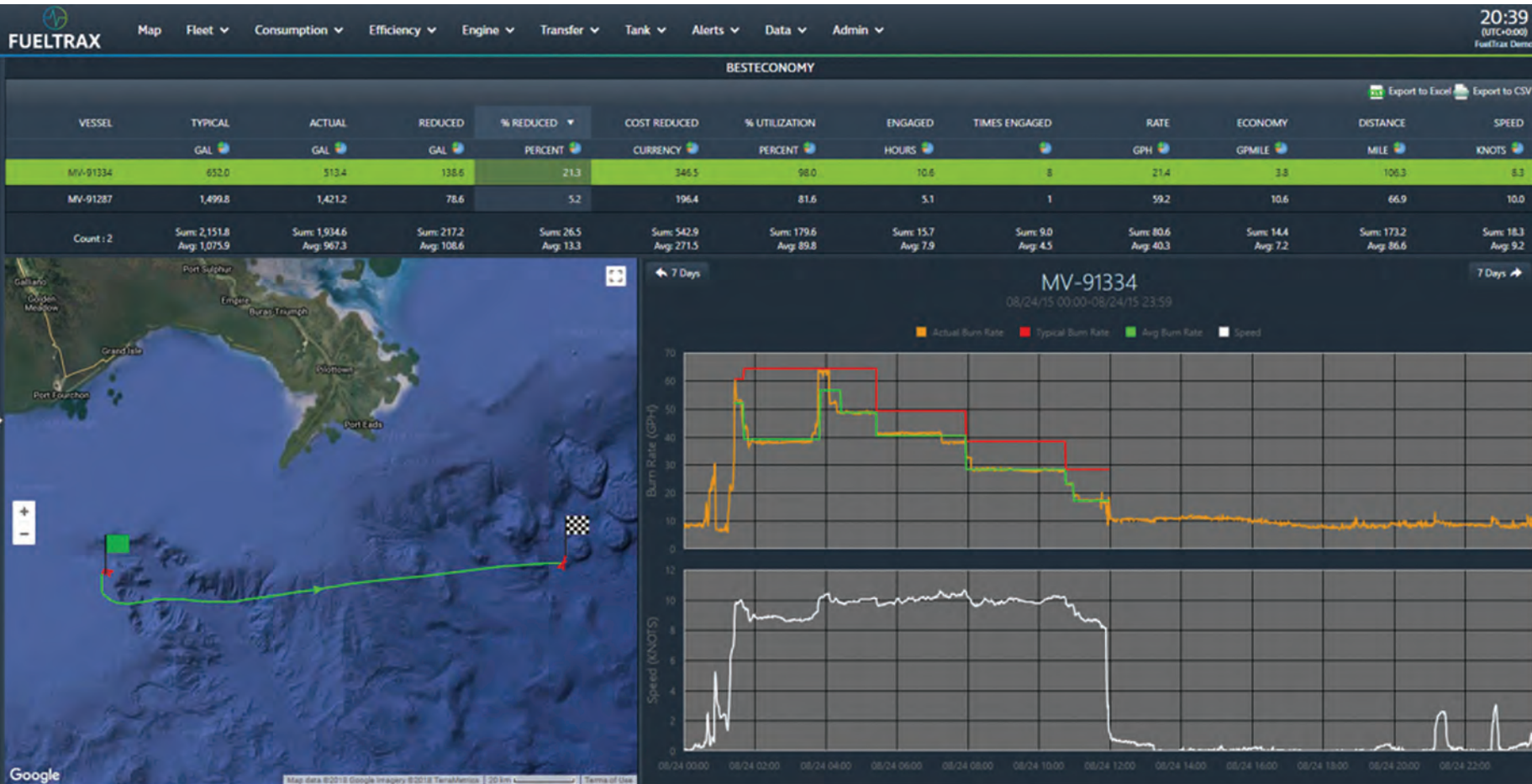
Figure 5. The BestSpeed algorithm recommended the optimal maximum speed with minimum fuel consumption, resulting in savings of 21.3% compared to the typical burn rate.
