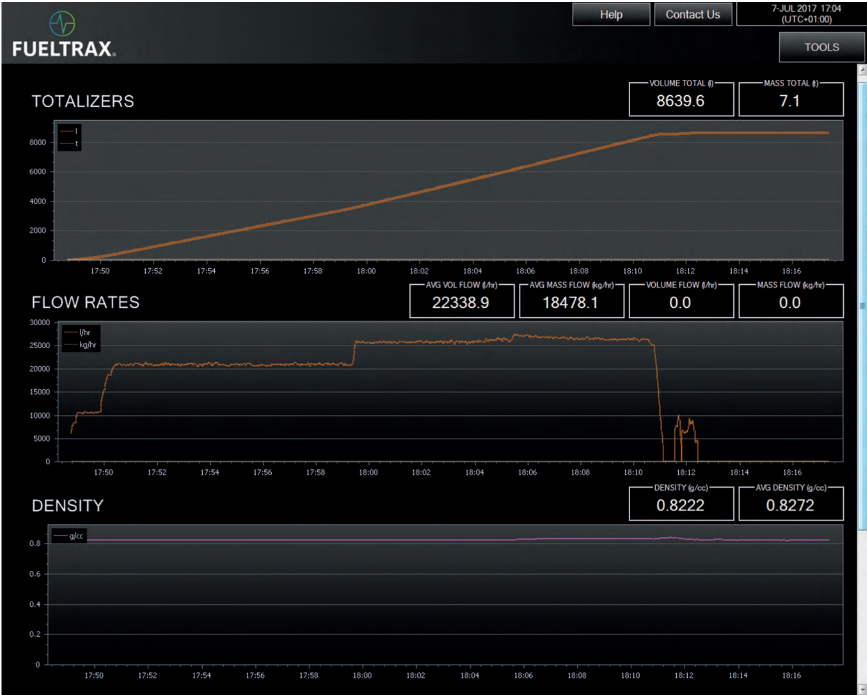
Figure 2. Endress+Hauser Coriolis mass flowmeters collect fuel consumption, density, temperature and other data—all of which are displayed onboard and transmitted to onshore facilities via satellite.
