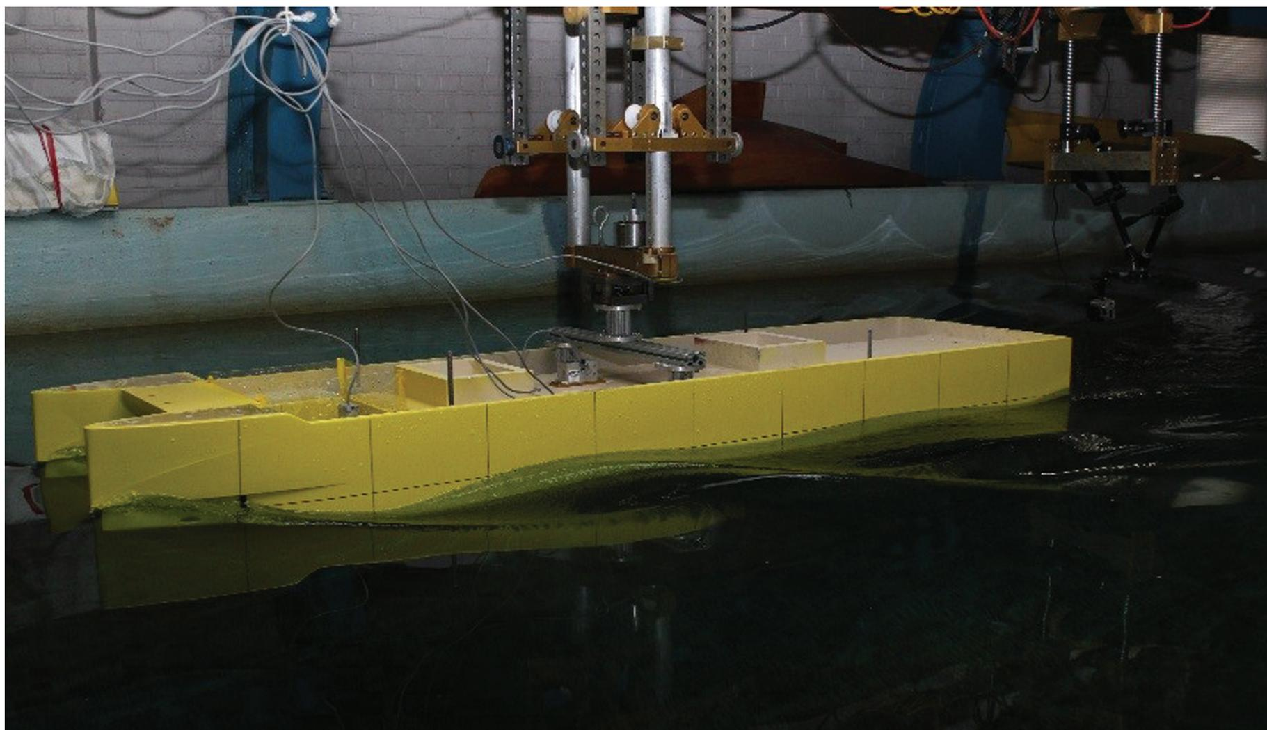
Figure 1: Resistance Testing
