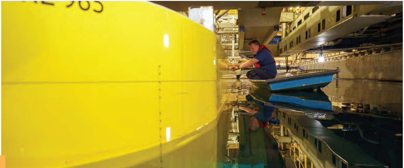
The Tow Tank @ NRC is a 200m (656 ft.) towing tank.
