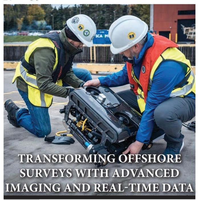
Technicians prepare an ROV equipped with a Rayfin Camera for an inspection.
