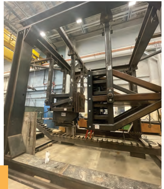
Inside the Structures Lab they can test the impact of ice on ship panels.
