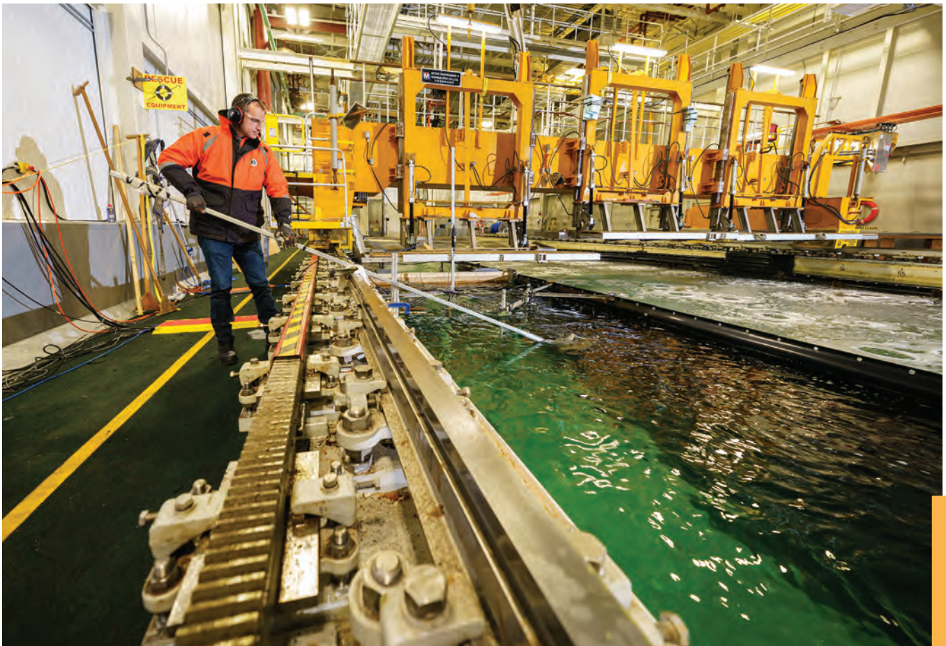
The World's Largest Ice Tank: The world's largest ice tank is 90m (295 ft.) long, and has been used to study dozens of challenges, including navigation and Arctic conditions and model tests of ice structure with temperatures that range to -25^{\circ}\text{C} ( -13^{\circ}\text{F} ).
