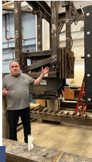
OERC has large structural testing equipment where it can test almost full-scale ship panels with ice, impacting 'ice' into the steel panels which represent a ship.
