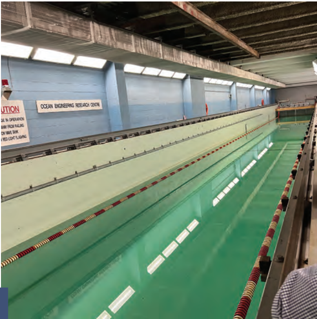
OERC's tow tank with a wavemaker, which is used for hydrodynamic studies into ships and offshore structures.
