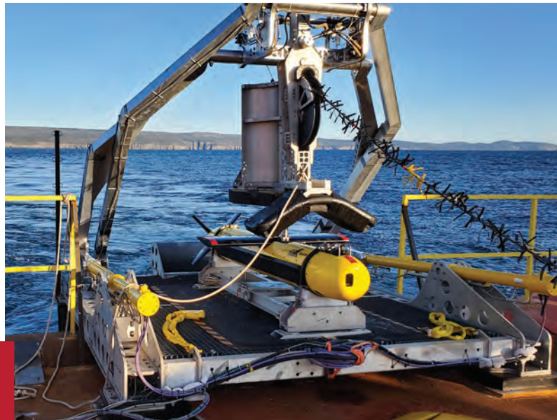
Kraken KATFISH towed synthetic aperture sonar system and autonomous launch and recovery system.
