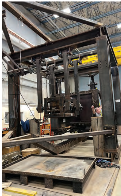
OERC has large structural testing equipment where it can test almost full-scale ship panels with ice, impacting 'ice' into the steel panels which represent a ship.
